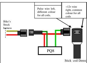
Suzuki GSXR, Hayabusa. Honda CBR. KTM, Superduke –07, RC8. (Superduke R 2008 uses Duc 749-1198 harness). RC-8 2011 and newer with 4 coils, connect green and blue coil wire pair to one cyl and yellow and brown to the other cyl.
